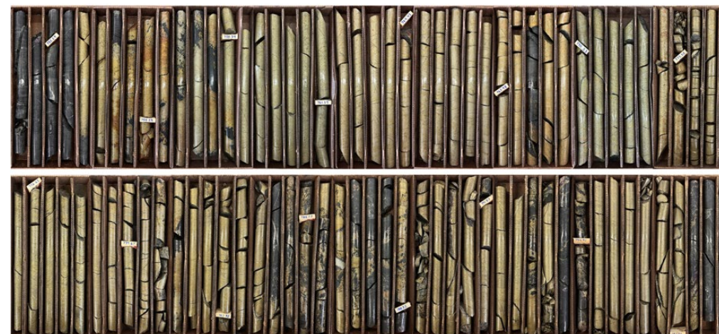
Drill core from drill hole 25TK0562A at 752.97 meters depth showing an interval of 46.43 meters of MSU and MMS.
