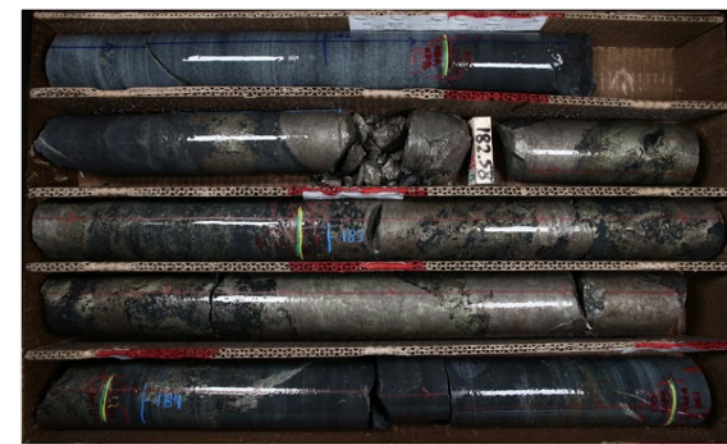
Hole 24BD0008 – 2.35m of nickel-copper massive sulphide mineralization.
