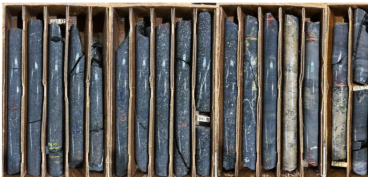
Figure 1: Drill core from hole 26RL0010 showing the lower portion of the intrusive conduit and the MSU interval near the footwall contact with the meta-sedimentary rock at approximately 594 meters.
