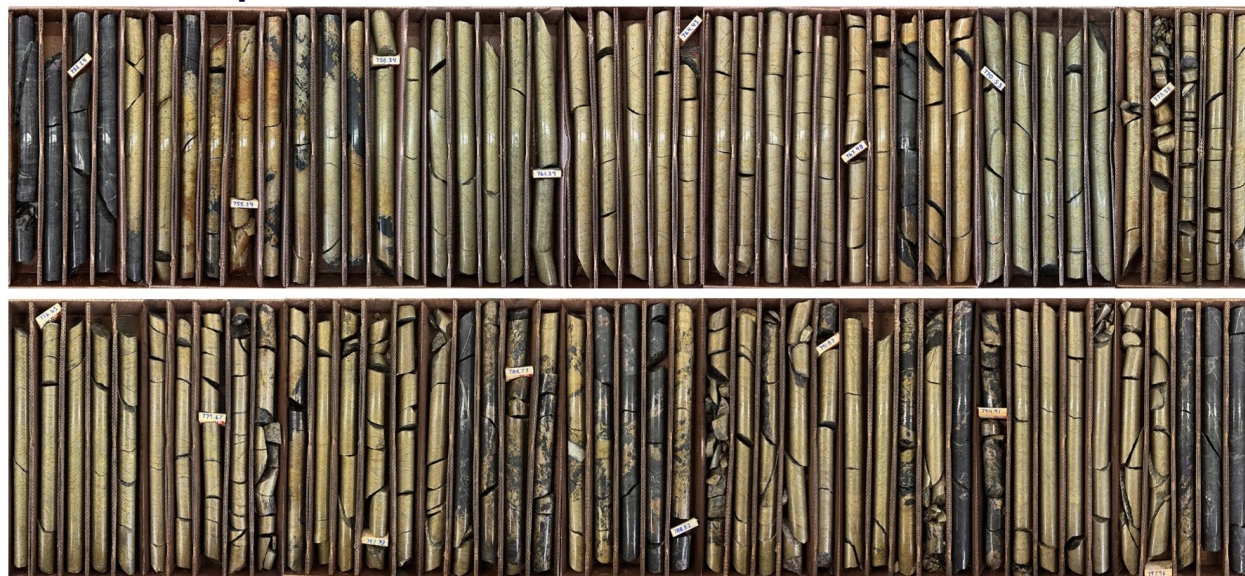
Figure 1: Drill core from drill hole 25TK0562A at 752.97 meters depth showing an interval of 46.43 meters of MSU and MMS.
