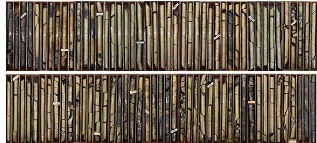
Drill core from drill hole 25TK0562A at 752.97 meters depth showing an interval of 46.43 meters of MSU and MMS (assays pending).
