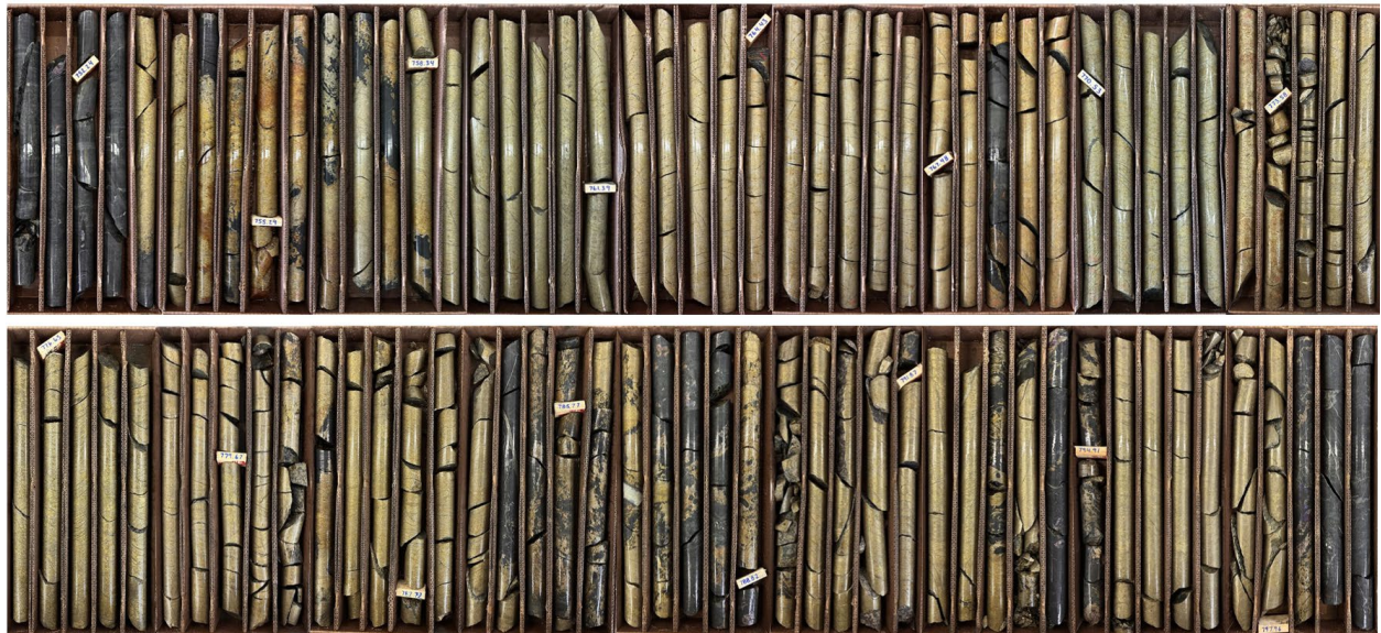
Figure 1: Drill core from drill hole 25TK0562A at 752.97 meters depth showing an interval of 46.43 meters of MSU and MMS.
