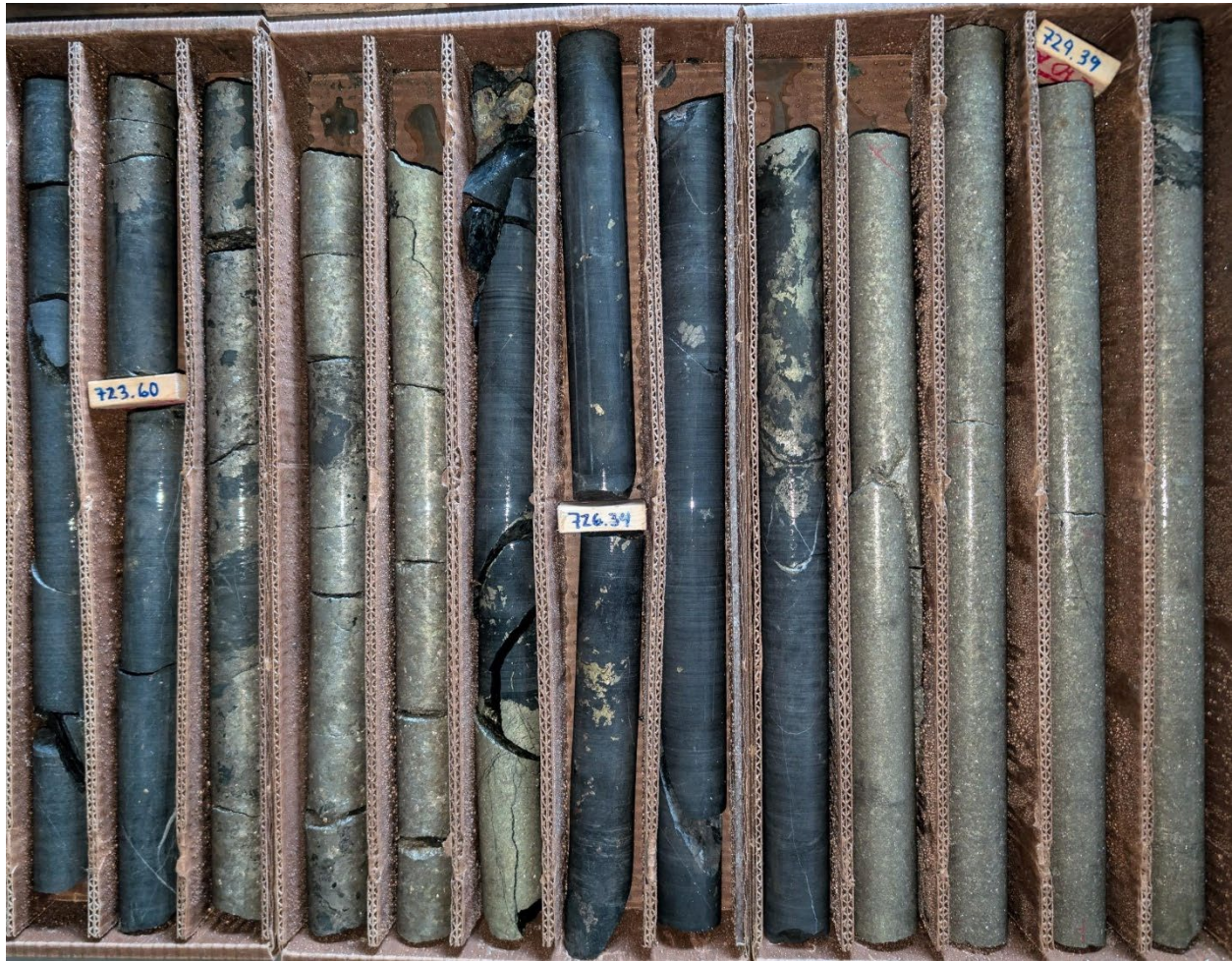
Figure 1: Drill core from hole 25TK0568C at the 710-meter level. Drill hole 25TK0568C intersected 7.20 meters grading 6.75% Ni, 7.50% Cu, 0.07% Co, 4.89 g/t Pt+Pd, and 2.32 g/t Au (12.27% NiEq or 23.42% CuEq) starting at 723.70 meters, including 2.50 meters grading 13.48% Ni, 12.05% Cu, 0.11% Co, 10.03 g/t Pt+Pd, and 4.75 g/t Au (22.48% NiEq or 44.97% CuEq) starting at 727.45 meters.
