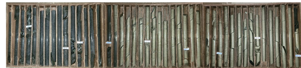
Photo of drill core from drill hole 25TK0563 at 762.34 meters depth showing a cumulative 34.9 meters of massive nickel mineralization.
