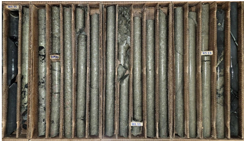
Photo of drill core from the extension of drill hole 16TK0250 at 707.75 meters depth showing 8.25 meters of massive sulphide grading 12.62% Ni, 13.88% Cu, 0.12% Co and 17.95 g/t PGEs+Au.
