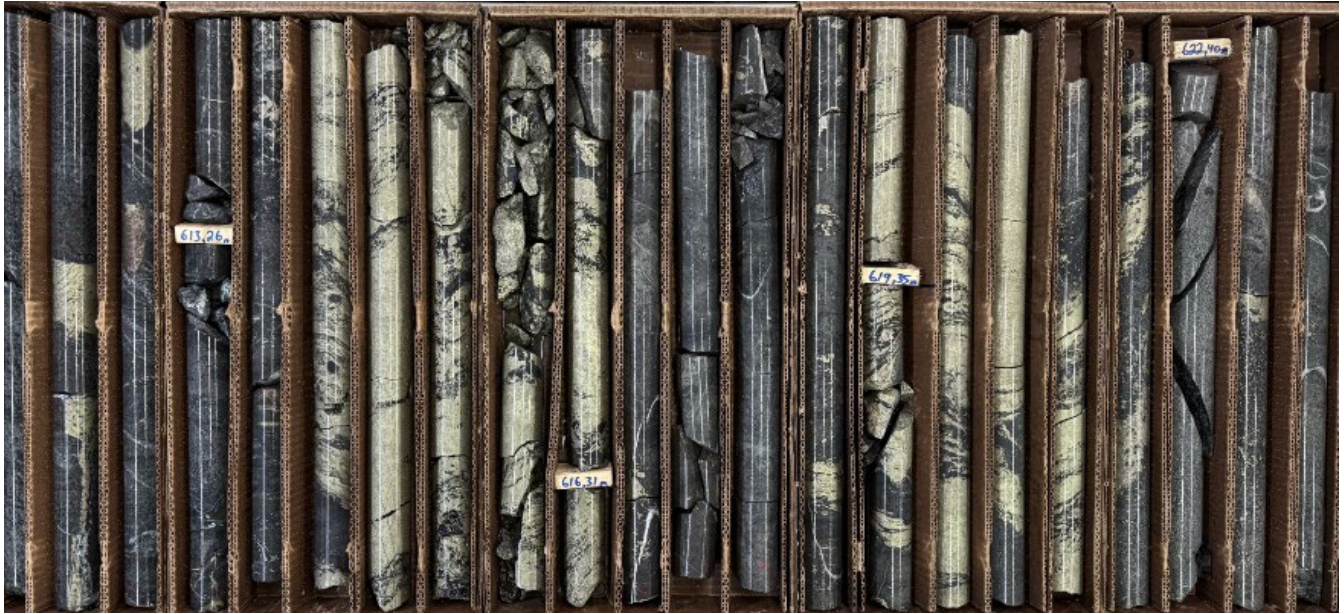
Figure 1: Drill hole 25TK0568 intercepted 10.35 meters of MSU/MMS interlayered with disseminated sulphides starting at 611.57 meters.
