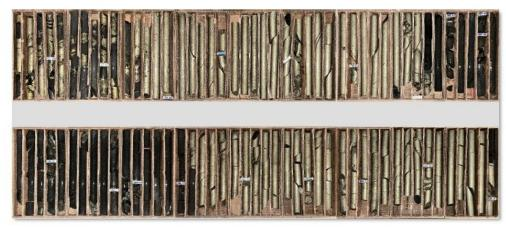
Photo of drill core from drill hole 25TK0563 at 762.34 meters depth showing a cumulative 34.9 meters of massive nickel mineralization
