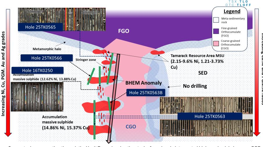
Conceptual cross-section through the Vault Zone showing the stack of previously intercepted high-grade nickel-copper-PGE mineralization. The near-vertical BHEM plate shown in Figure 1 (see conceptual placement) is interpreted to reflect a controlling structure for these known massive sulphides. The modelled conductor persists for hundreds of metres below the deepest intercept in drill hole 25TK0563
