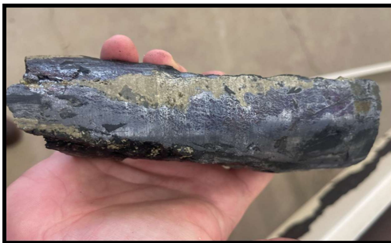
Figure 3: An example of massive chalcocite and bornite identified in hole 25TK0563A in the Vault Zone
