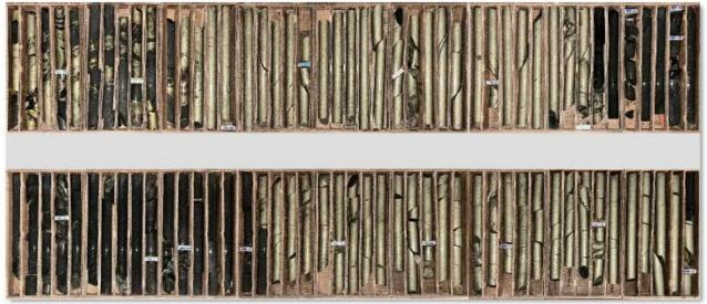
Photo of drill core from drill hole 25TK0563 at 762.34 meters depth showing a cumulative 34.9 meters of massive nickel mineralization
