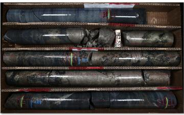
Hole 24BD0008 – 2.35m of nickel-copper massive sulphide mineralization
