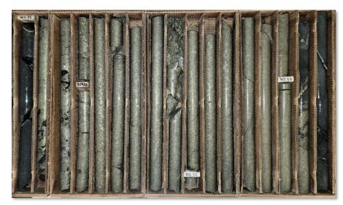
Photo of drill core from the extension of drill hole 16TK0250 at 707.75 meters depth showing 8.25 meters of massive sulphide grading 12.62% Ni, 13.88% Cu, 0.12% Co and 17.95 g/t PGEs+Au
