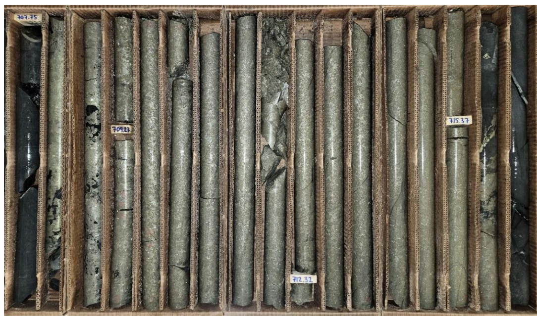
Figure 1: Photo of drill core from the extension of drill hole 16TK0250 at 707.75 meters depth showing 8.25 meters of massive sulphide
