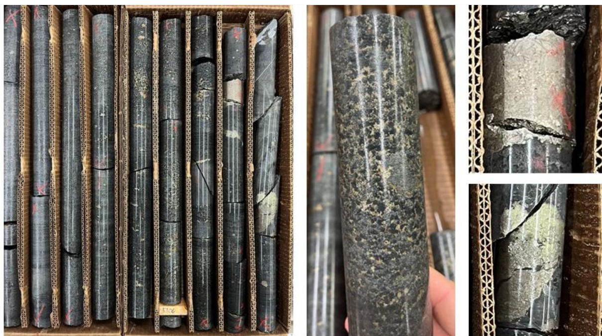
Figure 8: Three examples of new nickel-copper mineralization intercepted below the Tamarack Resource Area, with the center image showing net-textured nickel-copper mineralization and the right image showing massive sulphide nickel-copper mineralization (new drill hole 24TK0510).
