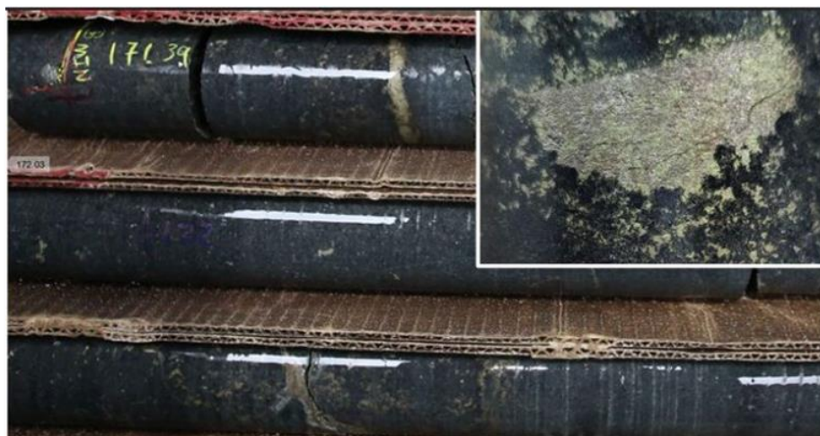
Figure 11: Core from drill hole 24BD0004 showing nickel copper massive sulphide veins which are often used to predict the existence of nearby massive sulphide. Inset image shows a massive sulphide rip up clast approximately 3cm in diameter.
