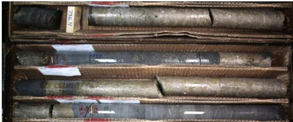
Figure 5: Drill core from 24TK0505 highlighting 1.8 meters of massive sulphide assaying 6.75% Ni, 3.06% Cu, and 2.15 ppm Pt+Pd+Au starting at 736.4 meters.
