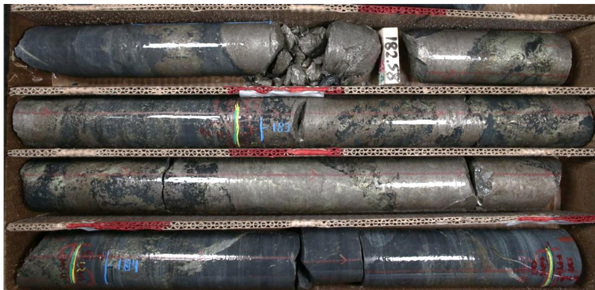
Figure 13: Core photo showing 2.09 meter thick interval of massive and mixed-massive sulphide starting at 182.34 meters depth in hole 24BD0008 at Boulderdash.
