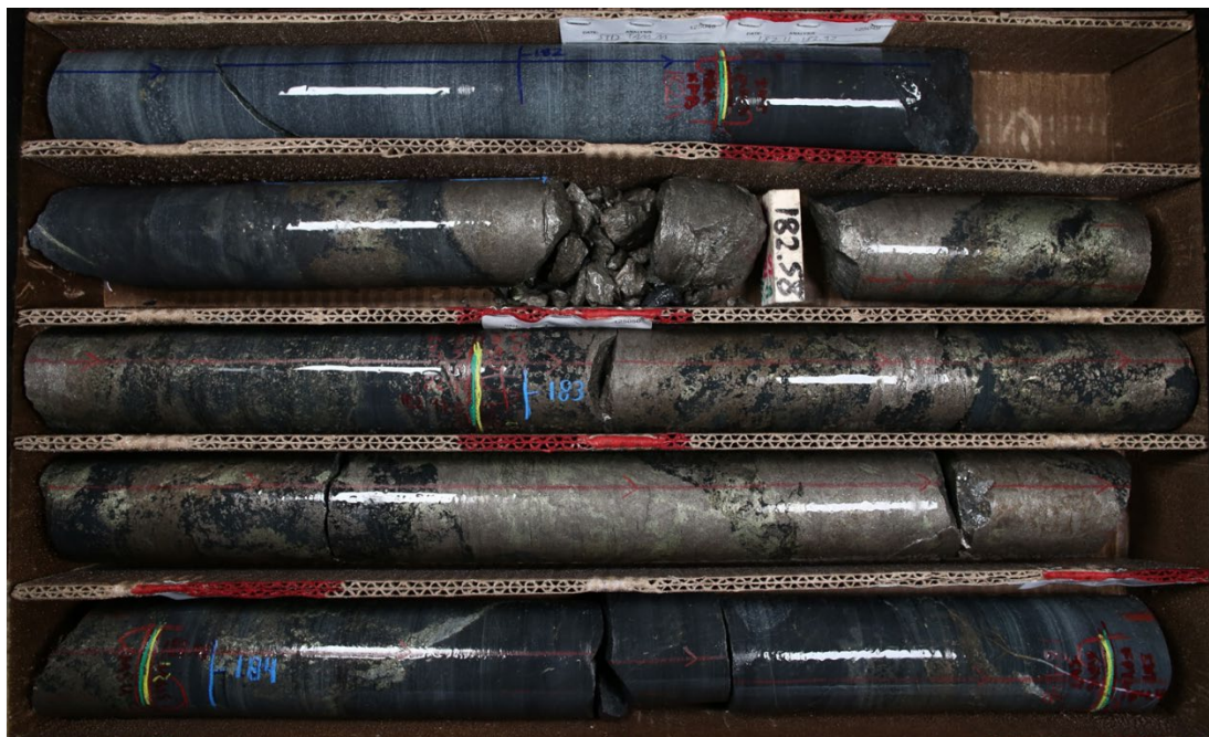
Figure 1: Photograph showing 2.35 meters of nickel-copper massive sulphide mineralization assaying 2.33% Ni and 2.95% Cu beginning at 182.11 meters depth in drill hole 24BD0008.
