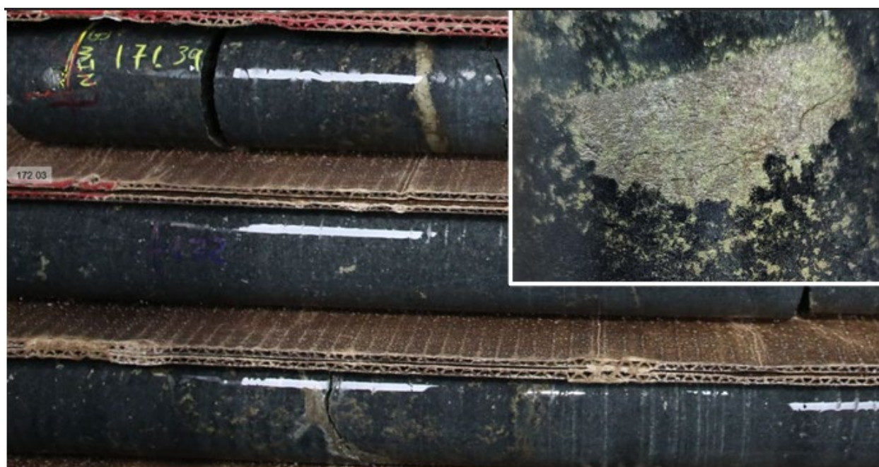
Figure 2: Core from drill hole 24BD0004 showing copper-nickel massive sulphide veins, which can often be used to predict the existence of a more significant accumulation of massive sulphide, and shows a Massive Sulphide Unit (MSU) clast identified approximately 3cm in diameter.
