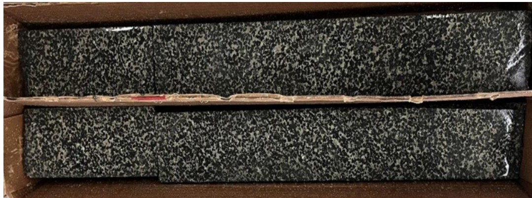
23TK0473 – 101.71m grading 3.04% NiEq (see August 21, 2023 press release)
