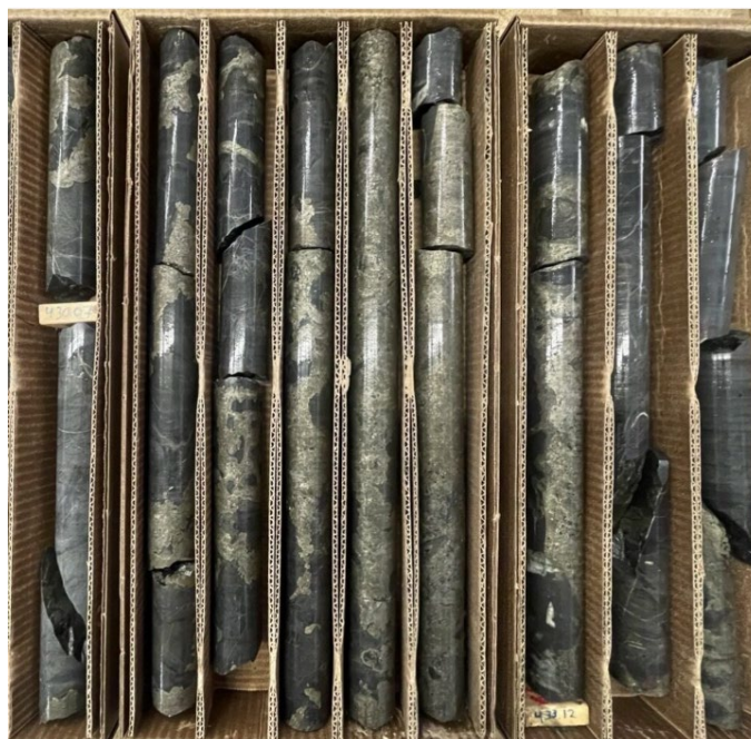
Figure 1: Drill hole 24TK0503 assayed at 4.89% Ni, 4.10% Cu, 0.06% Co, 4.10 Pd g/t, 6.19 Pt g/t, 7.16 Au g/t (9.26% NiEq) over 4.81 meters starting at 429.63 meters
