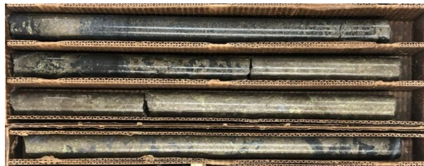
23TK0483 – 5.93m of 2.92% Ni and 1.73% Cu including 2.2m of 9.31% NiEq from 653m (see January 16, 2024 press release)
