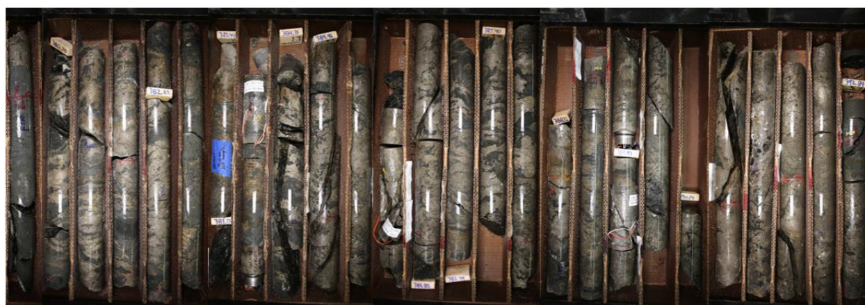
Figure 1: 12.72m assaying 7.5% NiEq intersected in drill hole 23TK0447 at a depth of 380 meters.
