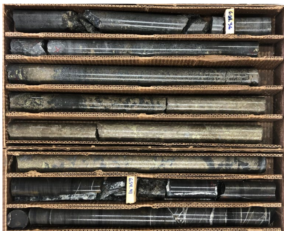
Figure 1: 2.2m of 9.31% NiEq intersected in drill hole 23TK0483 at a depth of 653 meters
