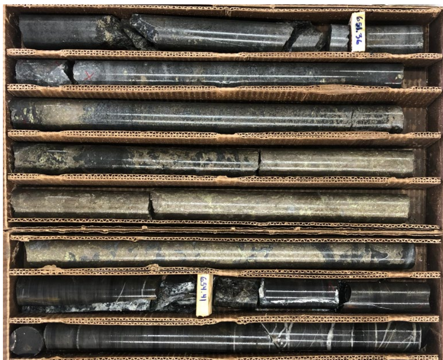
Figure 1: High-grade nickel and copper mineralization intersected in drill hole 23TK0483 at a depth of 653 meters
