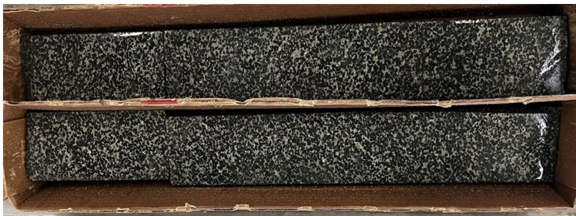
Figure 1: Portion of Drill Hole 23TK0473 that forms part of 101.71 meters (333 feet) of high-grade nickel-copper mineralization, grading 1.94% Ni, 1.84% Cu and 0.35 g/t Pd, 0.64 g/t Pt and 0.62 g/t Au (1.61 g/t PGEt + Au) (3.04% NiEq)
