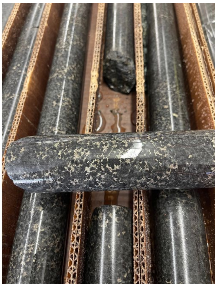
Figure 1: Nickel mineralization encountered between 296.03 and 298.7 meters depth in new drill hole 23TK0482
