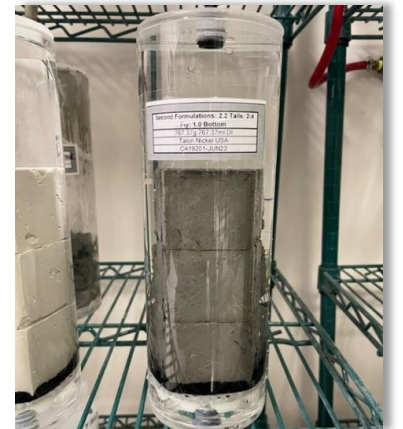
Fly ash/tailings blocks undergoing long-term chemical stability testing
