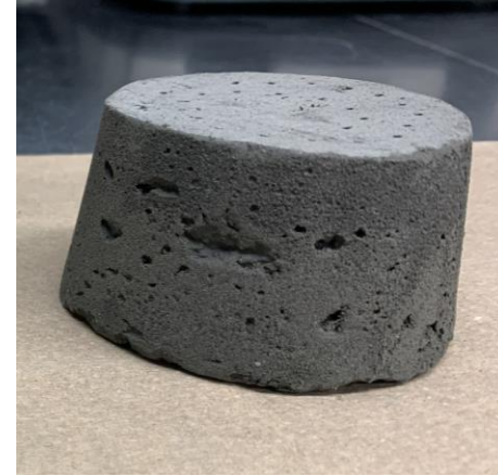
Fly ash/tailings mixture hardened into a solid block
