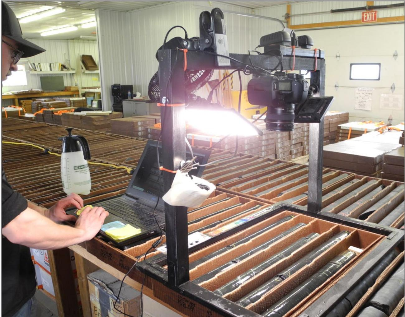
Note: The cm-scale and colour chart attached to the left side of the frame apparatus.
