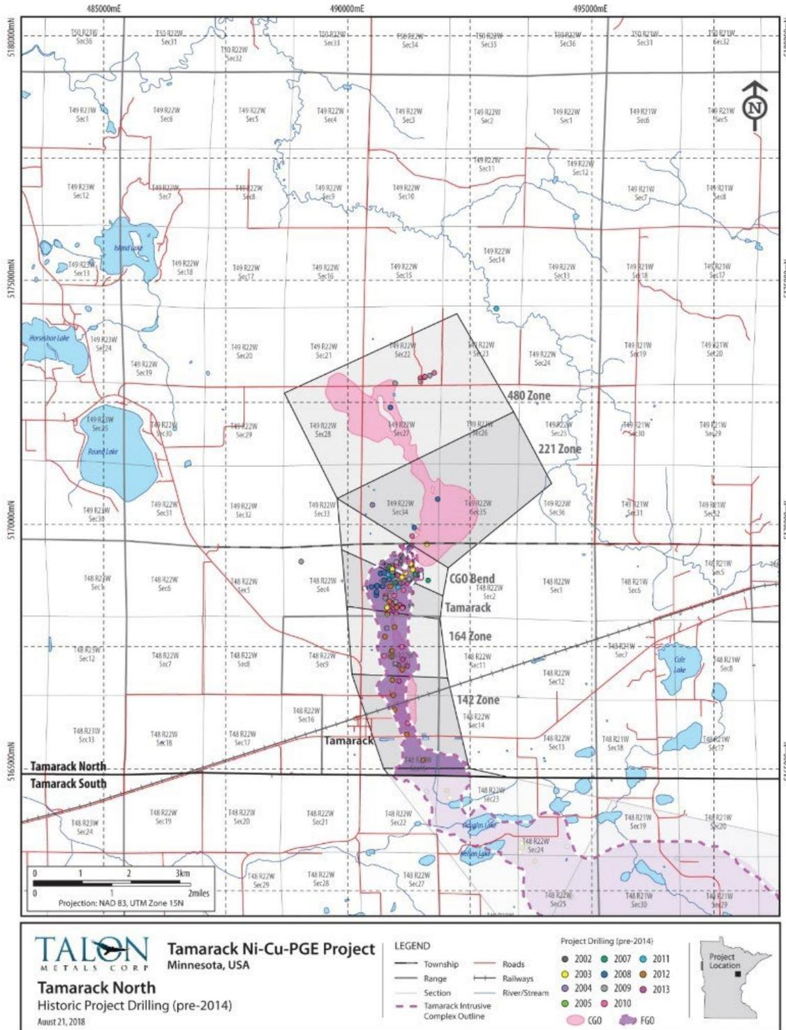
**Figure 6.2: Enlarged Map Showing Localities of Drill Holes, in the Tamarack North Project (background 1VD magnetic image). Modified from Kennecott Internal Report and Survey Data, 2013**
