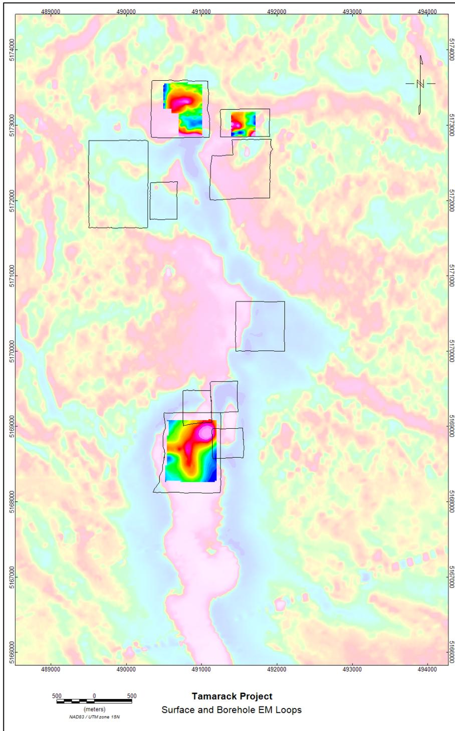
Note: The background image is the calculated vertical magnetic field from the compiled Tamarack airborne geophysical surveys.
