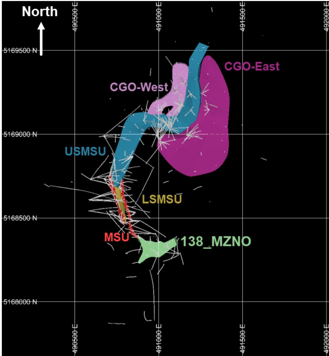
**Figure 14.2: Tamarack North Project Mineral Domains, with Drill Hole Traces in White; Oblique View Looking Northeast**
