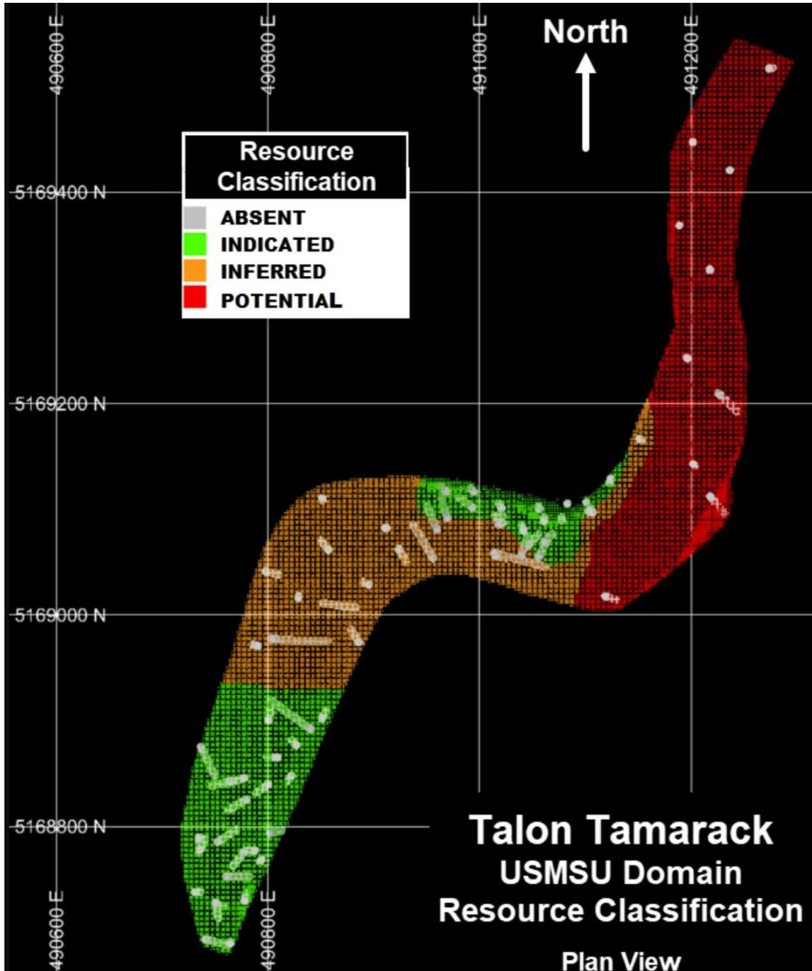
Figure 14.18: LSMSU Resource Classification, with Supporting Drill Hole Composited Samples as Gray Traces; Plan View
