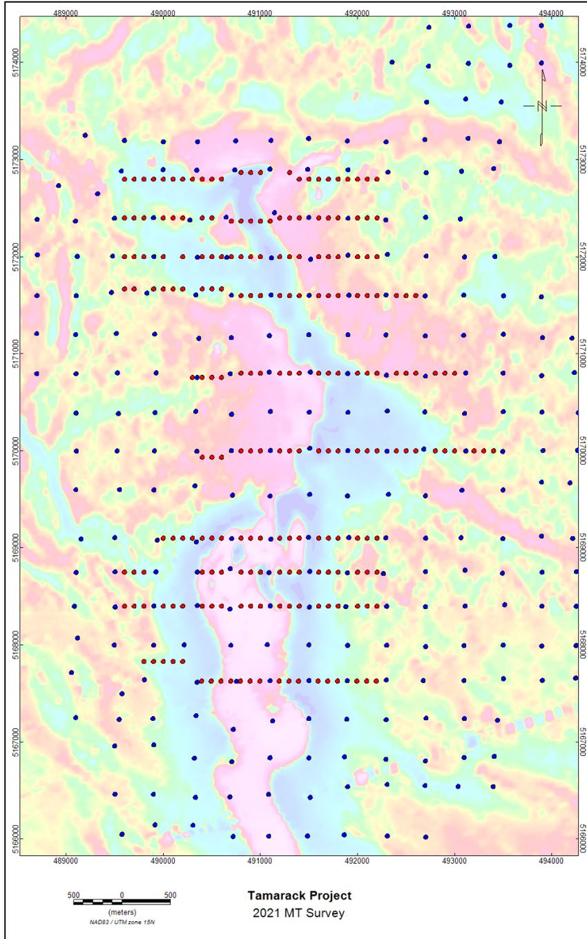
Note: The data is plotted over the calculated vertical gradient composite map generated after the Tamarack airborne EM campaigns. The 2021 infill survey covered from the Tamarack Main Zone to the North end of the known intrusion.
