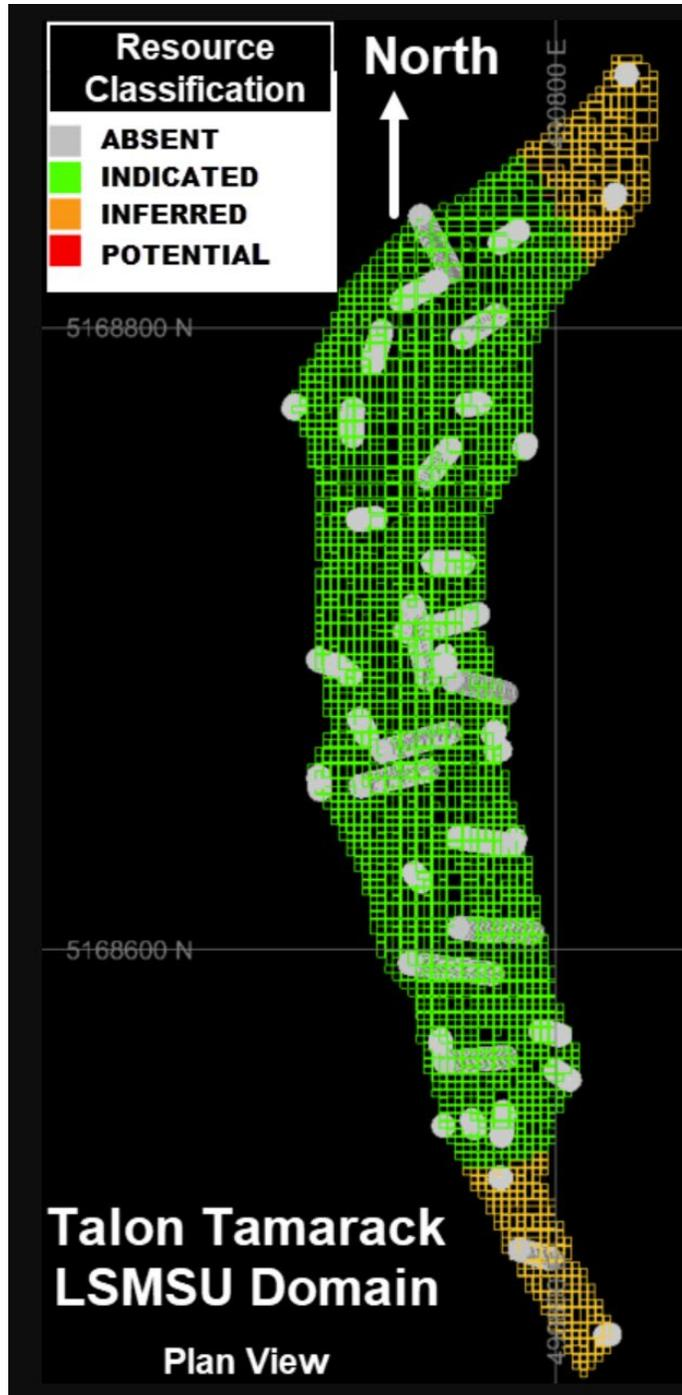
**Figure 14.19: MSU Resource Classification, with Supporting Drill Hole Composited Samples as Gray Traces; Plan View**
