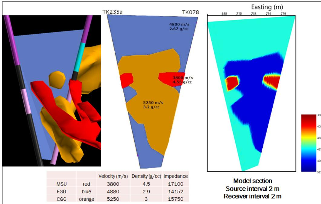
Note: A 2-dimensional section through the geologic model was created (left and centre) and the resulting tomographic data was simulated through this model. This simulated data was then inverted, resulting in the image on the right. The MSU appears to resolve as a distinct slowing anomaly displayed here in red.
