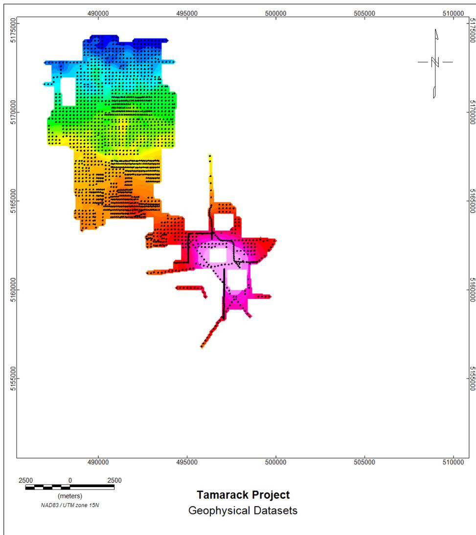
Note: Dots show locations of new data acquired in 2016 (Kennecott Gravity Survey, 2001, 2002, 2011, 2015 and 2016).
