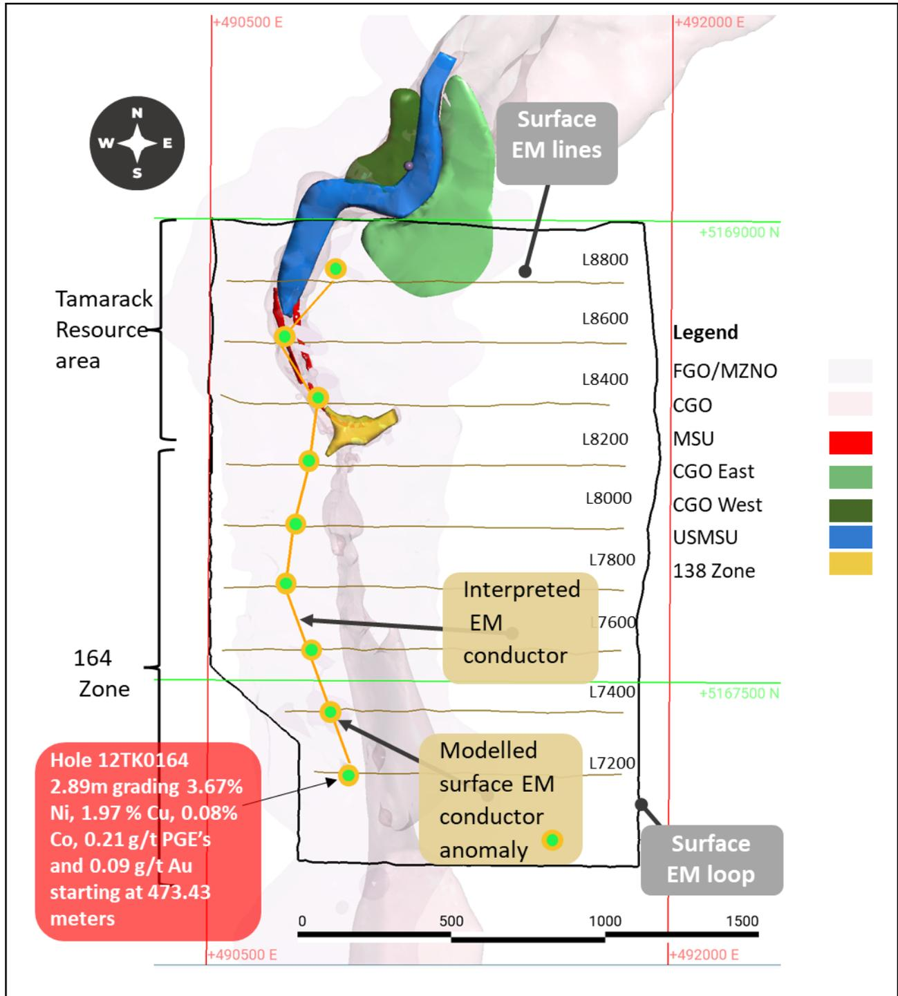
Note: The solid orange line shows the location of the interpreted conductive anomalies.
