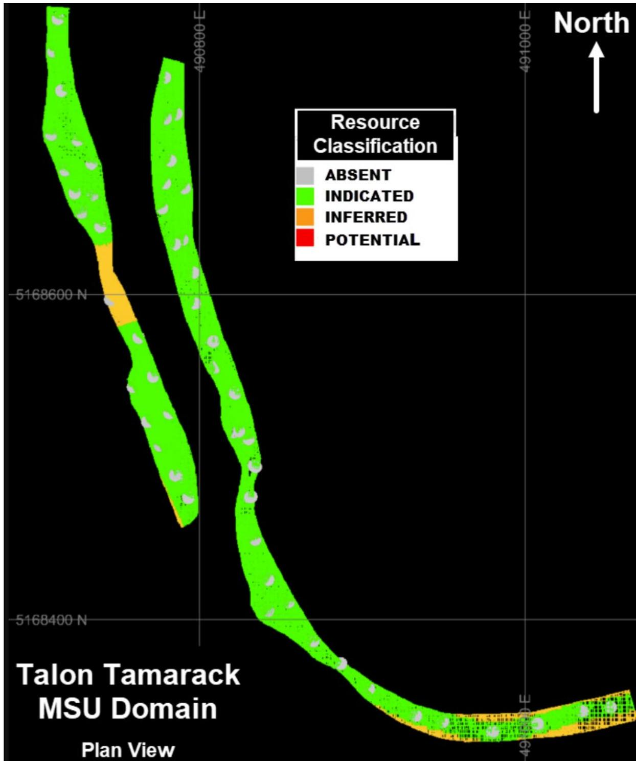
**Figure 14.20: 138 Zone Resource Classification, with Supporting Drill Hole Composited Samples as Gray Traces; Plan View**
