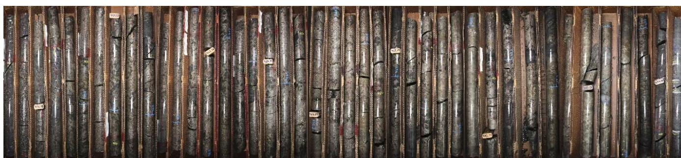
Figure 1: Drill core from hole 21TK0380 showing 23.44 meters of massive sulphide grading 6.04% Ni and 2.85% Cu from 453.73 meters depth in the Main Zone of the Tamarack resource area.
