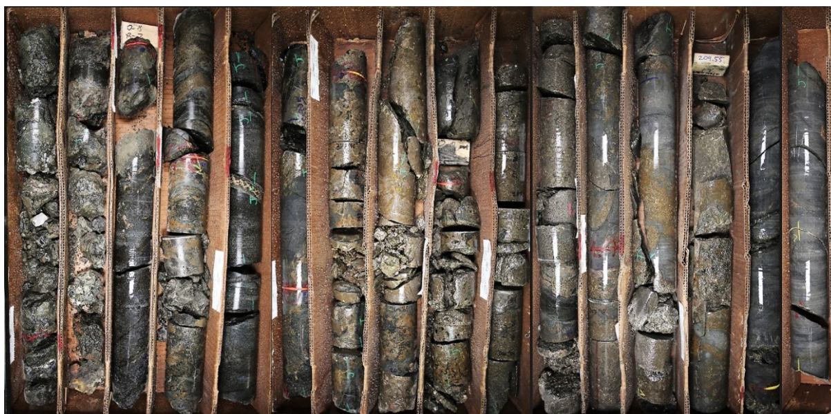
Figure 1: 4.89 meters grading 5.30% Ni and 2.27% Cu (6.51% NiEq or 17.37% CuEq) at 204.77 meters in drill hole 21TK0369
