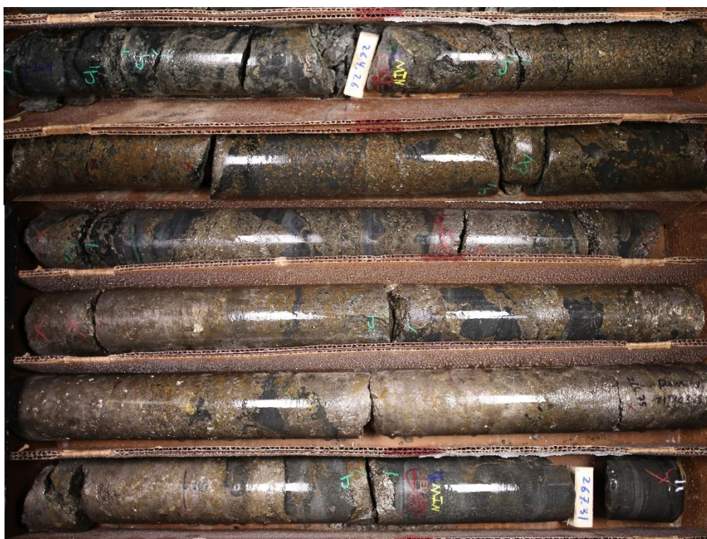
Figure 1: Drill hole 21TK0358 assayed 5.65% Ni, 2.04% Cu (6.88% NiEq, 18.36% CuEq) over 2.93 meters starting at 264.3 meters depth
