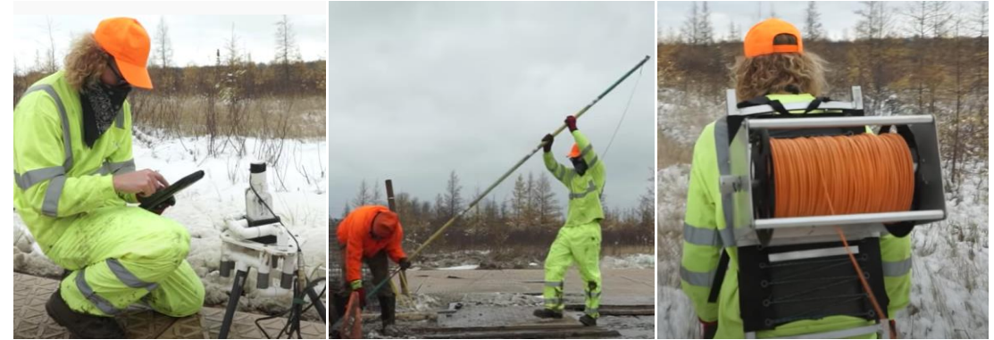
Geophysics – Surface and Borehole Electro-Magnetics surveys
