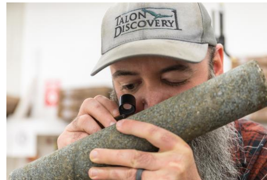
Talon geologists logging information including rock types, mineralogy and rock strength
