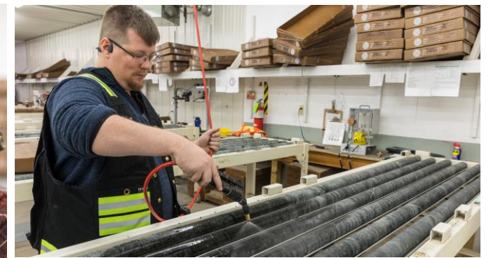
Talon geologists logging information including rock types, mineralogy and rock strength
