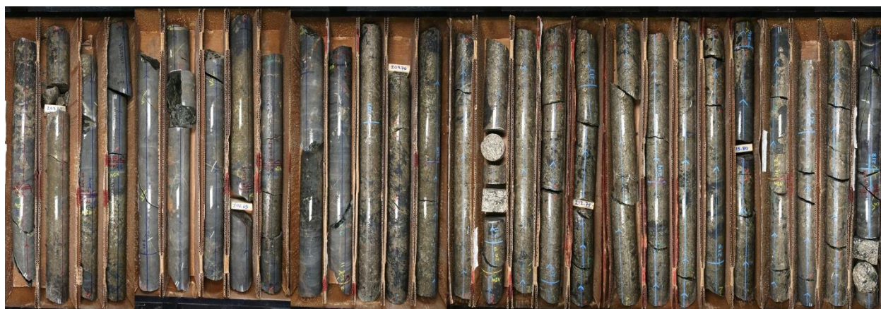
Figure 1: 15.08 meters of mixed and massive sulphide nickel and copper mineralization in 21TK0355 beginning at 202.86 meters depth
