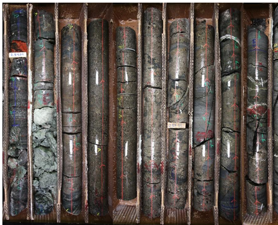
Figure 1: Drill hole 21TK0311 assayed 3.50% Ni, 1.40% Cu (4.38% NiEq, 11.68% CuEq) over 4.35 meters starting at only 234.5 meters depth
