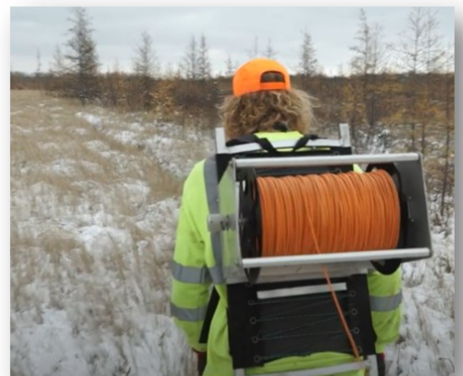
Bob Kryzer, Geologist, collecting surface Electro-Magnetic (EM) survey data to help identify drill targets.
