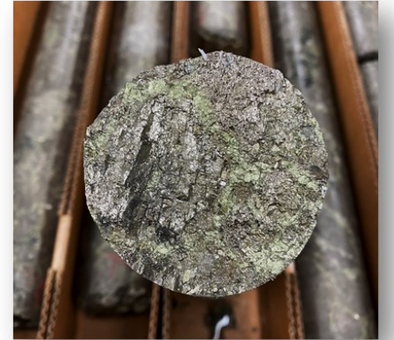
Sample core from the Tamarack Nickel Project Massive Sulphide Nickel Mineralization
