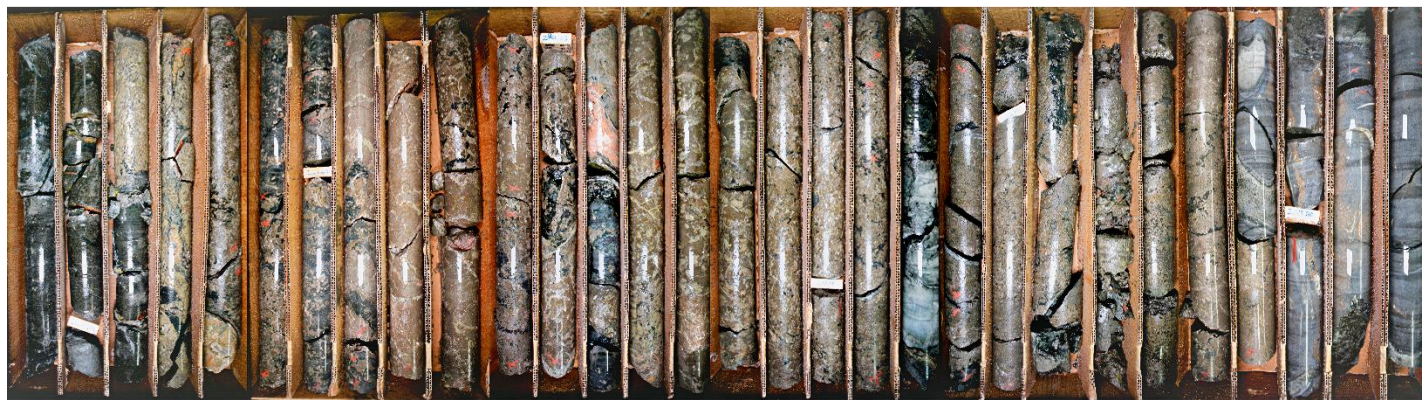
Figure 1: 13.92 Meters (45.5 feet) of massive nickel-copper sulphide mineralization in drill hole 21TK0313 assaying 5.54% Ni, 2.14% Cu (6.7% NiEq or 17.86% CuEq) drilled outside of the Tamarack Nickel Project’s resource area (in the CGO West Area)
