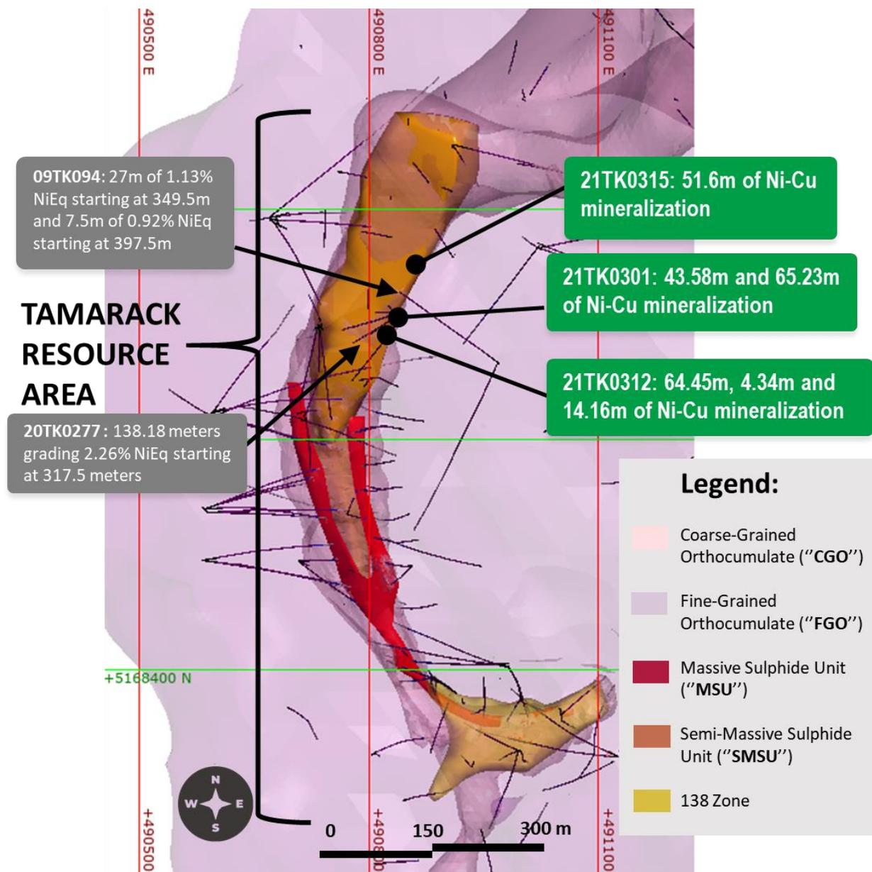
Figure 2: Plan view geological map of the Tamarack Nickel Project's resource area showing the location of new drill holes 21TK0301, 21TK0312 and 21TK0315.
