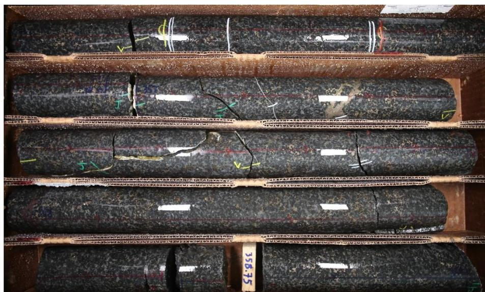
Figure 1: Portion of new drill hole 21TK0301, representing 2.77 meters (9.09 feet) of nickel-copper mineralization starting at 356.24 meters.
