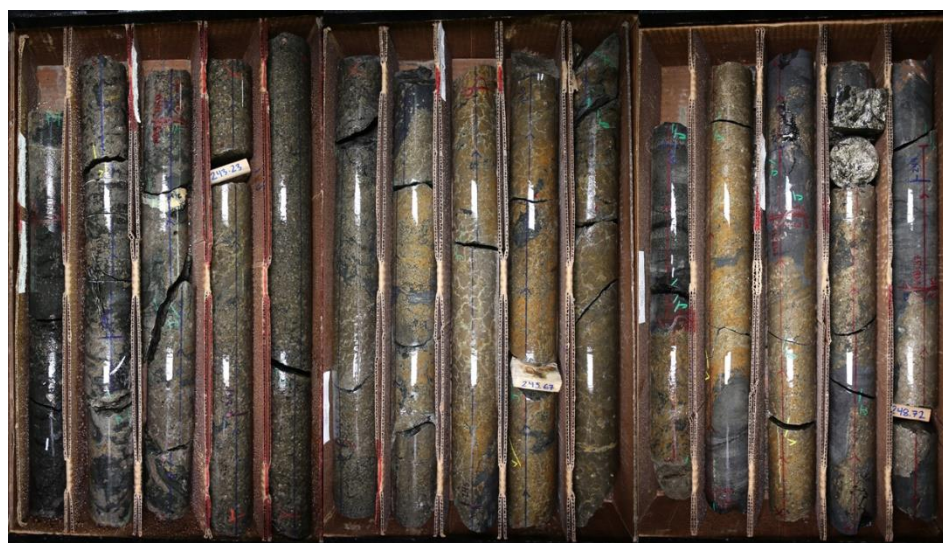
Figure 1: 7.31 meters (23.6 feet) of mixed massive nickel-copper mineralization in drill hole 21TK0316 from the CGO West area
