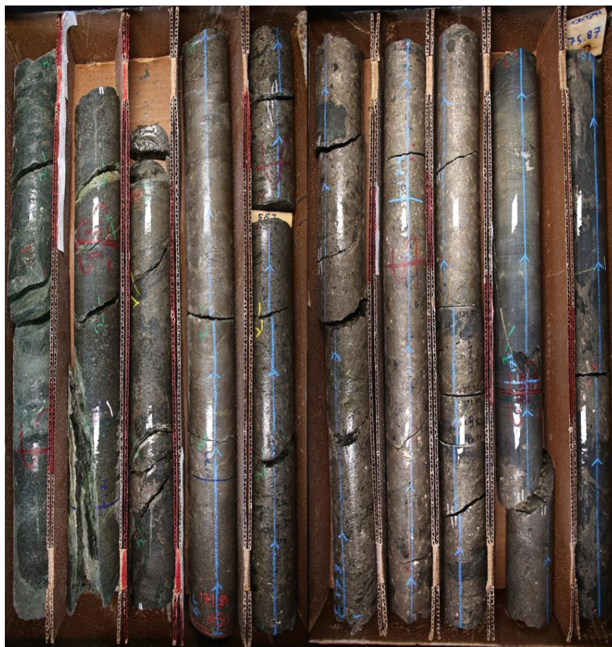
Figure 1: 5.1 Meters (16.7 feet) of massive sulphide mineralization at 171 meters depth grading 4.99% Ni, 1.66% Cu, (6.03% NiEq or 16.09% CuEq) in Drill Hole 21TK0283
