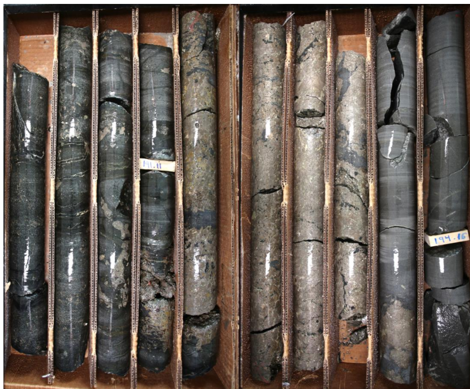
Figure 1. 2.28 meters (7.5 feet) of massive sulphide nickel mineralization grading 5.86% Ni, 2.35% Cu, 0.18% Co, 0.27 g/t Pd, 0.45 g/t Pt and 0.28 g/t Au (7.21% NiEq or 19.23% CuEq) starting at 191.32 meters (Drill Hole 21TK0287)
