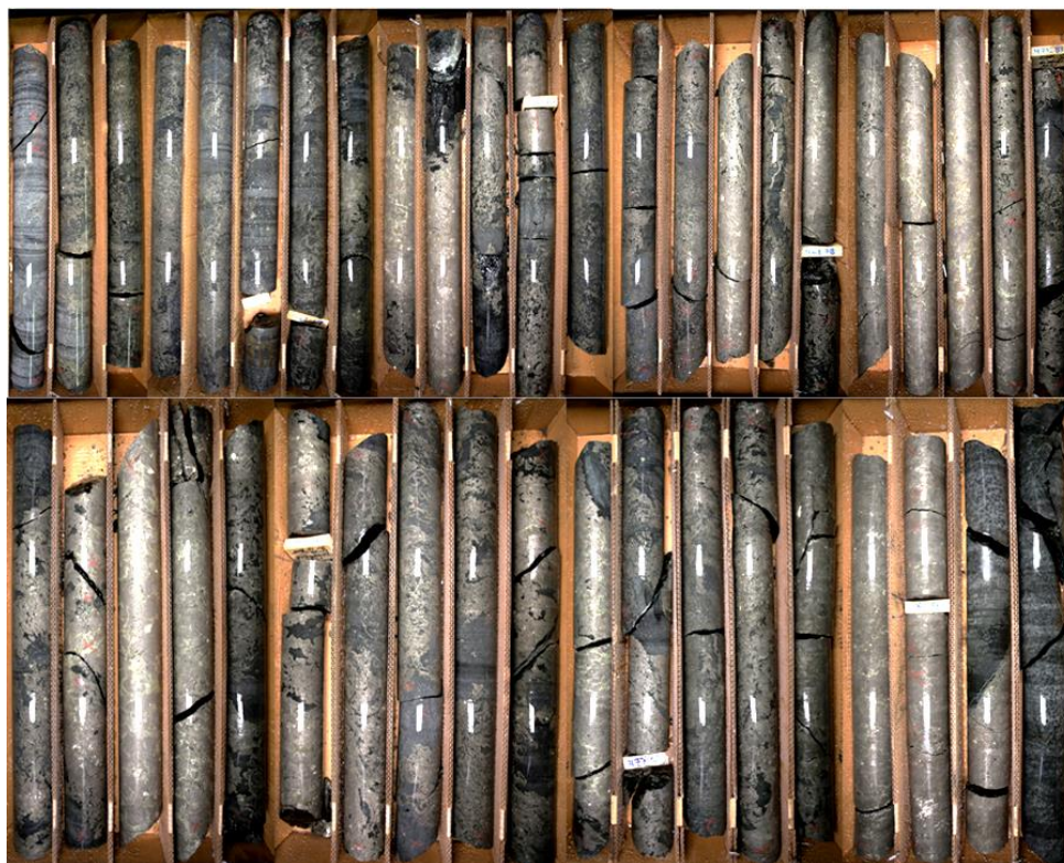
Figure 1: 21.73 Meters (71.2 feet) of Mixed Massive Sulphide Mineralization grading 6.72% Ni, 2.95% Cu, 0.13% Co, 0.56 g/t Pd, 0.76 g/t Pt and 0.38 g/t Au (8.35% NiEq or 22.28% CuEq) starting at 459.72 meters. (Drill Hole 20TK0278)
