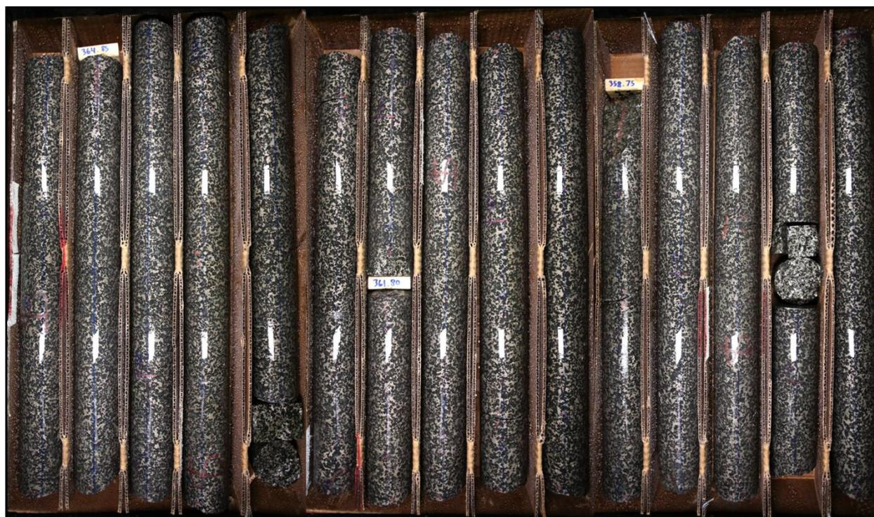
Figure 1: Portion of Drill Hole 20TK0277, representing 39.03 meters (128 feet) of semi-massive sulphide mineralization starting at 347.15 meters (Drill hole 20TK0277)
