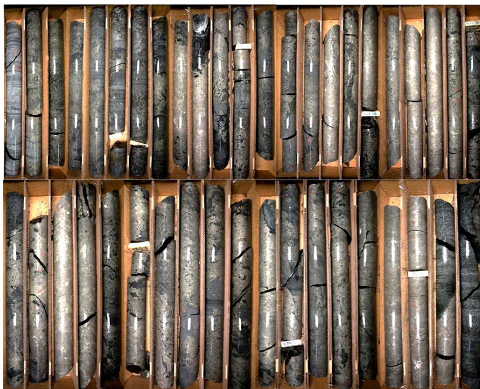
Figure 1: 21.73 meters (71.2 feet) of mixed massive sulphide mineralization starting at 459.72 meters (Drill hole 20TK0278)
