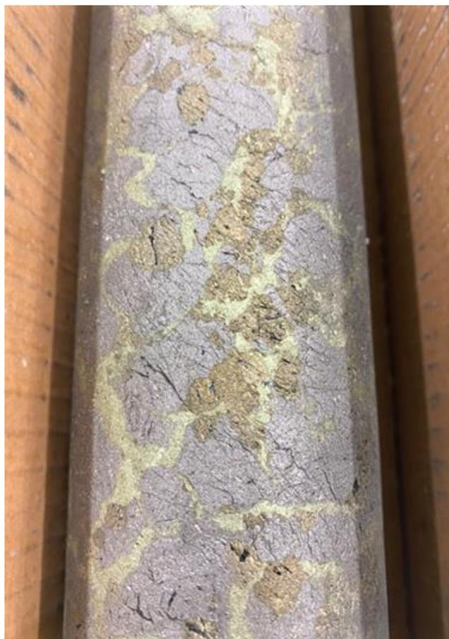
**Figure 2: Sample from drill hole 20TK0278 showing the loop textures with large pentlandite eyes**
