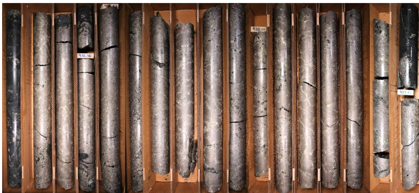
Figure 1: 8.39 meters (27.53 feet) of massive sulphide mineralization grading 8.15% Ni, 3.01% Cu, 0.19% Co, 0.54 g/t Pd, 0.62 g/t Pt and 0.17 g/t Au (9.83% NiEq or 26.21% CuEq), starting at 414.73 meters (Drill hole 20TK0273)
