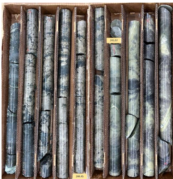
Figure 1: 2.71 meters (8.9 feet) of massive sulphide mineralization grading 5.13% nickel starting at 242.84 meters (Drill hole 20TK0271)
