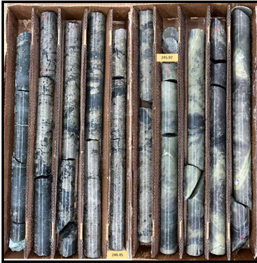
FIGURE 1: MASSIVE SULPHIDE MINERALIZATION STARTING AT 242.84 METERS (Drill hole 20TK0271)
