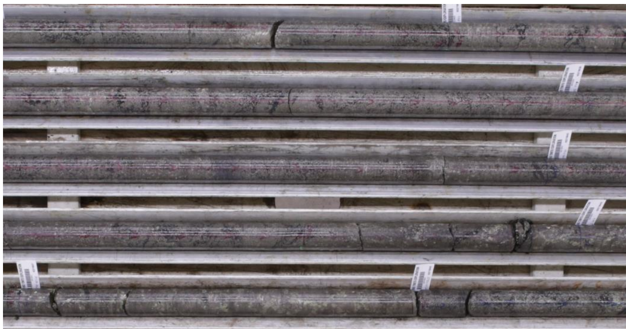
Figure 5: Core photo of massive nickel-copper-PGE sulphide mineralization intercept in hole 14TK0211.
