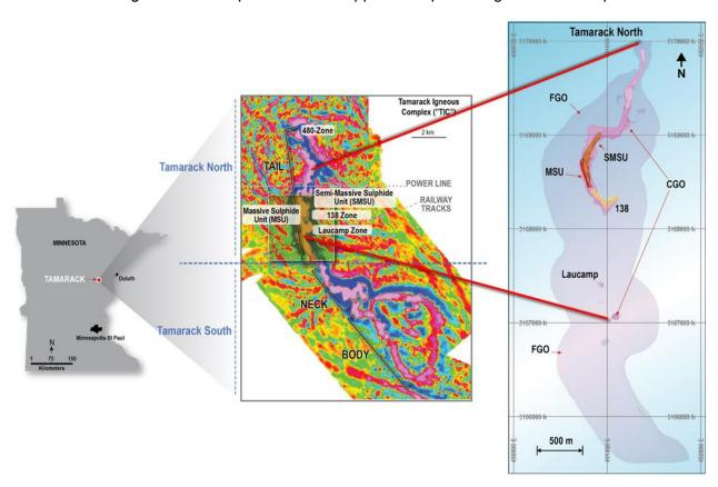
Figure 3: Airborne magnetic survey, first derivative image (centre) showing the 18 km long strike of the TIC with the long narrow intrusion that hosts the currently defined mineralization (right) termed the "Tail" of the Tamarack North Project and the large layered intrusion to the south termed the "Neck" and "Body" (in an analogy to a tadpole). Kennecott Airborne Magnetic Survey (2001 to 2009), modified by Talon, 2014.
