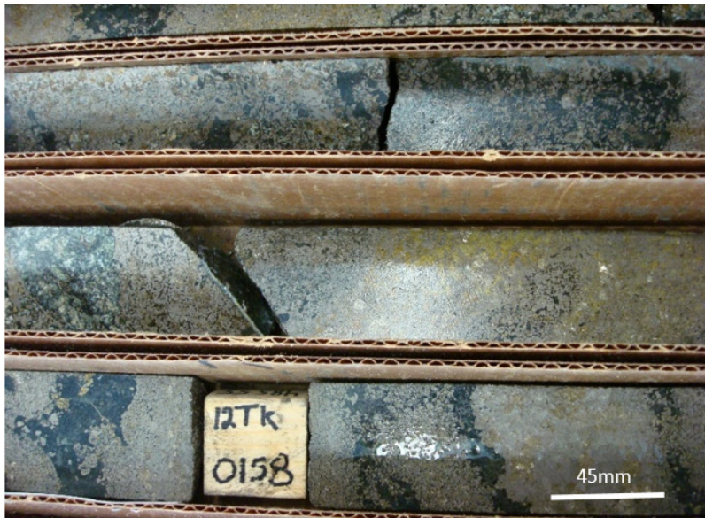
Figure 7-10: MSU from Tamarack Drill Hole 12TK0158
