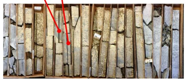
Figure 2: Image showing Metasediment and Mixed Massive Sulphide (MMS) units from drill hole 13TK0171, from 573.3m to 580.8 meters depth
