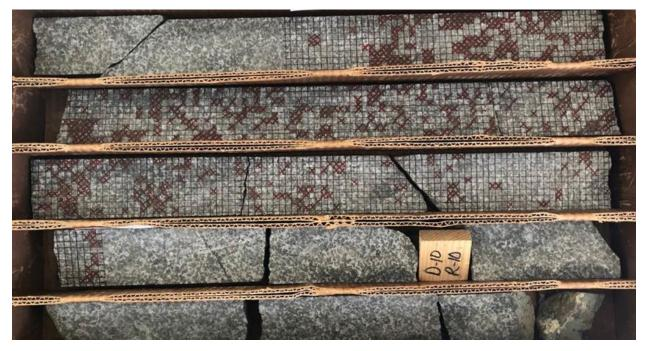
Figure 3: 1.5m sample interval, from 406m depth to 407.5m depth in drill hole 16TK0242, was broken down into a  $\frac{1}{4}$ " grid and marked where sulphide minerals were visually observed
