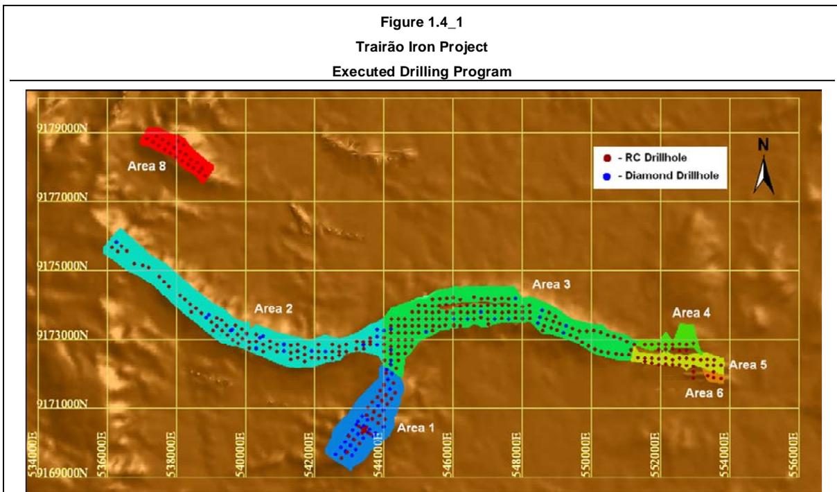
The entire drilling program, including RC and diamond drilling, comprised a total of 33,714 metres (Table 1.4\_1). RC drilling tested all the 13 target areas while diamond drilling was concentrated on Target Area 1, 2 and 3.
